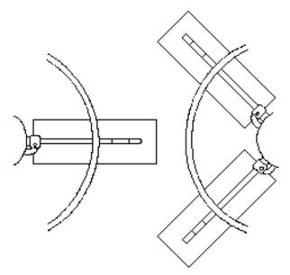
To avoid blades hitting, make sure spider plates are positioned as shown with respect to each other after performing any maintenance.
